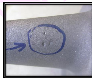
FOD on leading edge of bucket
